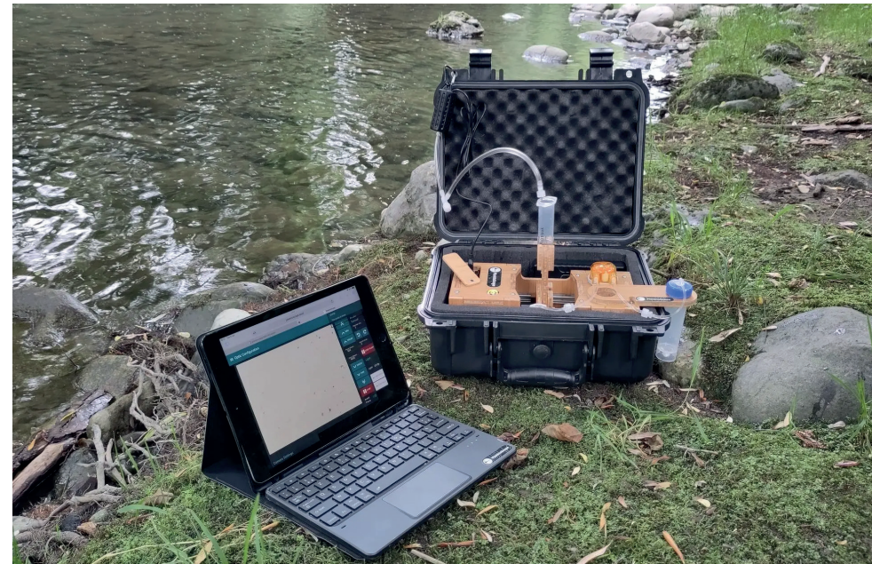
[15] Planktoscope in use on the banks of a body of water (FairScope, n.d.)
