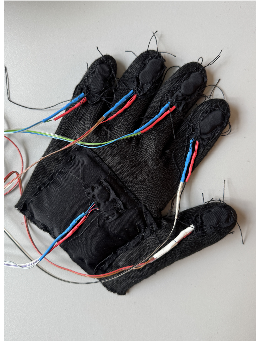
[59] Haptic Gloves prototype (May 2026)
